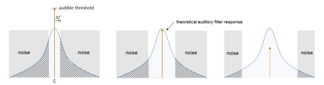
The notched-noise method assumes the audible threshold corresponds to a constant signal-to-masker ratio at the output of the theoretical auditory filter. That is, the ratio of the power of the  $f_c$  tone and the shaded area is constant. Therefore, the relationship between the audible threshold and  $2\Delta f$  (the notch bandwidth) is linearly related to the relationship between the noise passed through the filter and  $2\Delta f$ .
