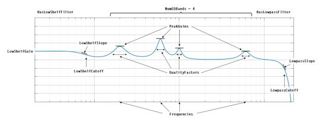
To implement a multiband parametric equalizer:
