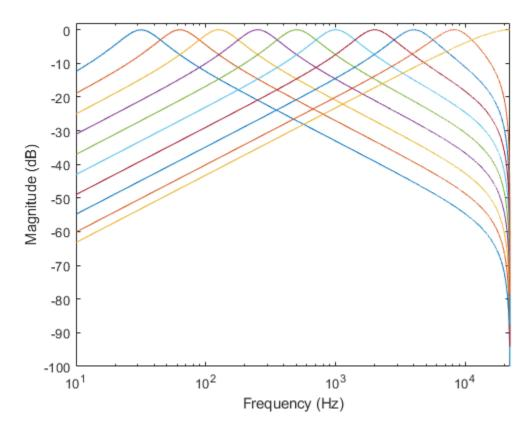
To visualize the magnitude frequency response only, call freqz without any output arguments. Plot the magnitude frequency response, in dB, of filters 4, 5, and 6 using a 1024-point DFT.
