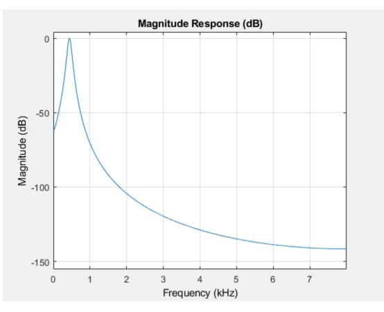
To specify the number of FFT points used to compute the frequency response, use the NFFT name-value pair. Specify that the frequency response is calculated using a 8192-point FFT.
