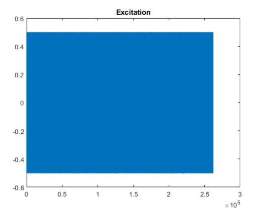
Replicate the excitation signal four times to measure the average of three measurements. The recording of the first MLS sequence does include all the impulse response information, so impzest discards it as a warmup run. Pad the excitation signal with zeros to account for the filter latency.
