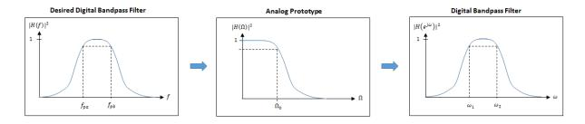
1 The analog Butterworth filter is expressed as a cascade of second-order sections:  $H(s) = H_1(s)H_2(s)\cdots H_{2N}(s),$
