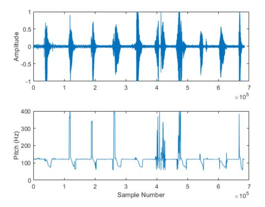
The pitch function estimates the fundamental frequency of the input signal at locations determined by the WindowLength and OverlapLength name-value pairs.
