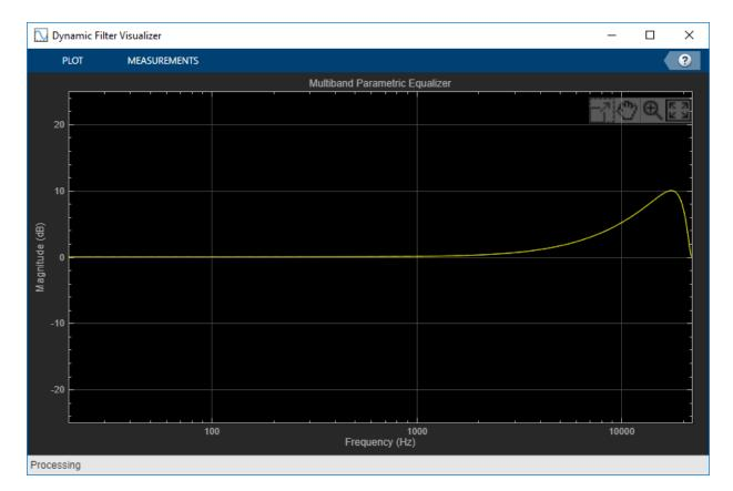
The equalizer band is warped.
