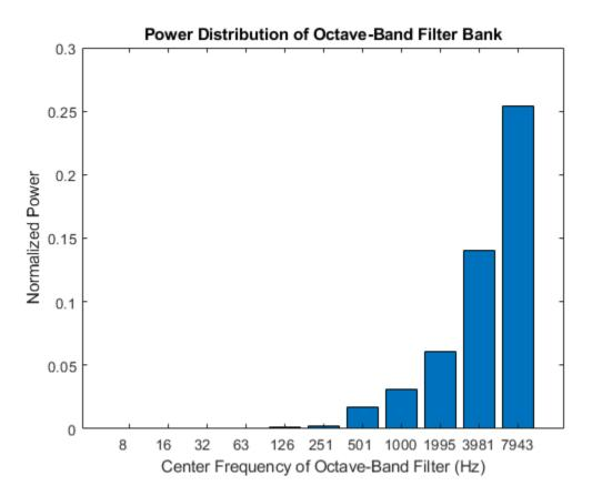
The band power increases by a factor of approximately two because the octave bandwidth increases by a factor of two. The power distribution of an octave filter bank mimics how higher frequencies are perceived louder in white noise. You can use octave filter banks to weight a spectrum for perceived loudness.
