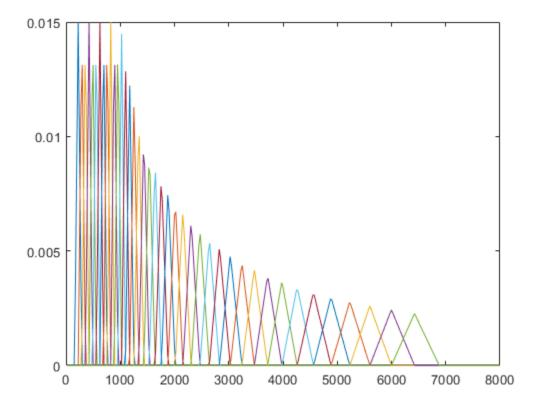
All the band edges are below the Nyquist frequency, and the bandpass filters in the filter bank have nonzero coefficients.
