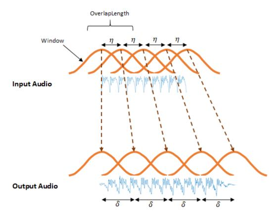
The OLA algorithm does a good job of recreating the magnitude spectra but can introduce phase jumps between windows. The WSOLA algorithm attempts to smooth the phase jumps by searching <code>WSOLADelta</code> samples around the  $\eta$  interval for a window that
