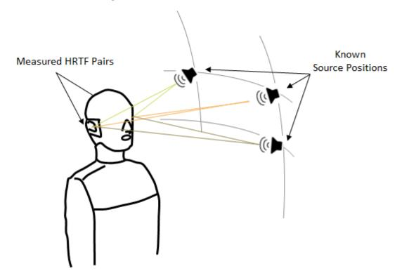
If you specify HRTF with real numbers, the function assumes that the input represents an impulse response, and *M* corresponds to the length of the impulse response. If you specify HRTF with complex numbers, the function assumes that the input represents a transfer function, and *M* corresponds to the number of bins in the frequency response. The output of the interpolateHRTF function has the same complexity and interpretation as the input.
