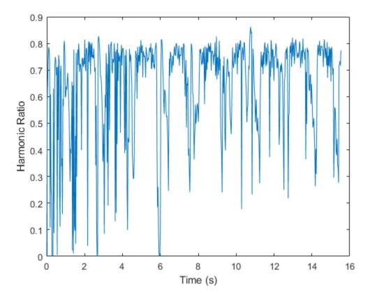
The harmonic ratio indicates the ratio of energy in the harmonic portion of audio to the total energy of the audio. Because the audio signal in this example has regions of near silence, where the total energy is very low, the harmonic ratio does a poor job discriminating between regions of speech and regions of silence. Add white noise to the audio signal and then calculate and plot the harmonic ratio.
