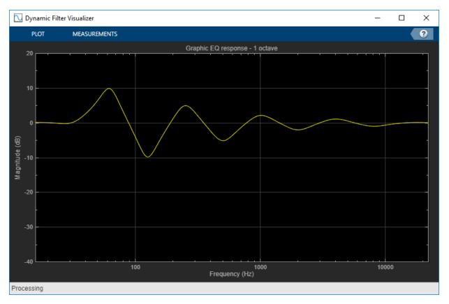
Call parameterTuner to open a UI to tune parameters of the equalizer while streaming.
