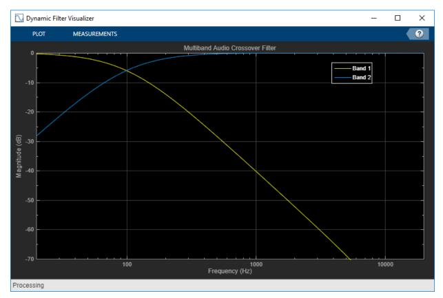
Call parameterTuner to open a UI to tune parameters of the crossover filter while streaming.
