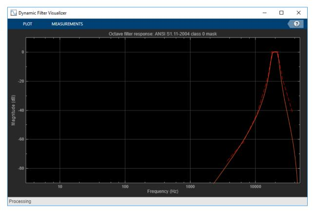
The red mask on the plot defines the bounds for the magnitude response of the filter. The magnitude response of this filter goes above the upper bound of the compliance mask
