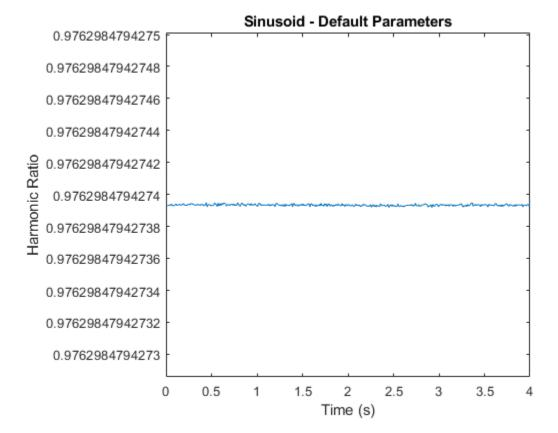
The short-time analysis required for windowing lowers the harmonic ratio from the theoretical value of 1. To diminish the effect of windowing, you can increase the window size. Use a 100 ms Hamming window and a 10 ms hop, and observe that the harmonic ratio is closer to one than when using the default window length.
