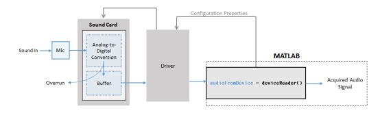
See "Audio I/O: Buffering, Latency, and Throughput" for a detailed explanation of the audio device reader data flow.
