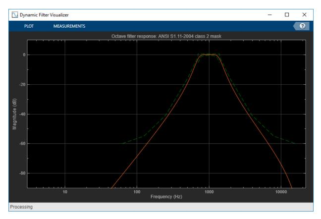
Analyze the filter using fvtool.
