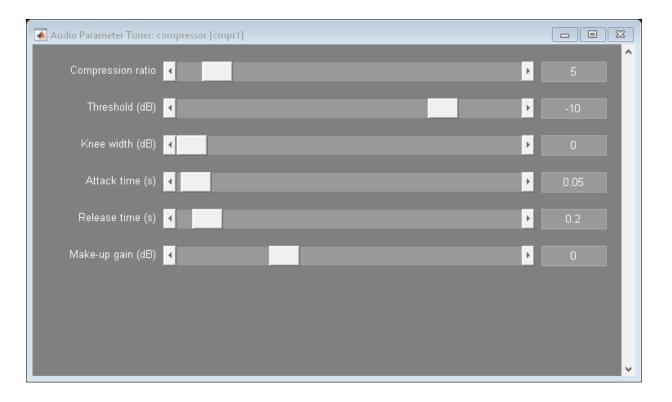
cmpr2 = compressor('SampleRate',fileReader.SampleRate); visualize(cmpr2) parameterTuner(cmpr2)
