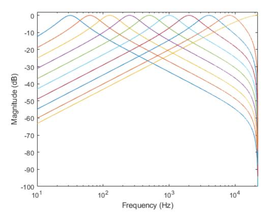
To get the frequency response of a subset of filters in the filter bank, specify the second argument as a row vector of indices between one and the number of filters in the filter bank. Get the frequency response of the 5th filter in the filter bank and plot the magnitude frequency response in dB.
