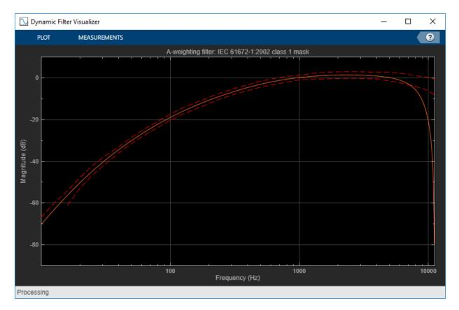
Change your A-weighting filter sample rate to 44.1 kHz. Verify that the filter is standard compliant and visualize the filter design.
