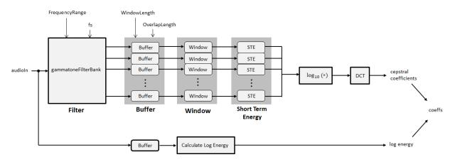
The FrequencyRange and sample rate (fs) parameters are set on the filter bank using the name-value pairs input to the gtcc function. The number of filters in the gammatone filter bank is defined as hz2erb(FrequencyRange(2)) -
