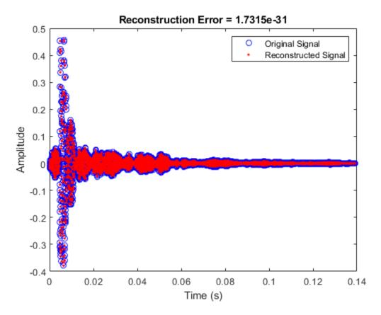
You can perform the MDCT and IMDCT without input padding using the PadInput namevalue pair. However, there will be a reconstruction error in the first half-frame and last half-frame of the signal.
