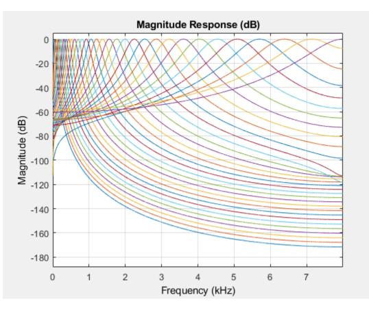
To visualize a subset of filters in the filter bank, specify the second argument as a row vector of indices between one and the number of filters in the filter bank. If not specified, fvtool visualizes 1 to N filters of the filter bank, where N is the smallest of gammaFiltBank.NumFilters and 64. Visualize the ninth filter.
