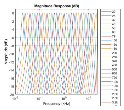
Process white Gaussian noise through the filter bank. Use a spectrum analyzer to view the spectrum of the filter outputs.
