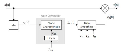
**1** The *N*-point signal, *x*[*n*], is converted to magnitude:
