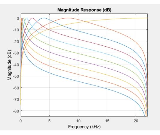
To visualize a subset of filters in the filter bank, specify the second argument as a row vector of indices between one and the number of filters in the filter bank. If not specified, fvtool visualizes 1 to N filters of the filter bank, where N is the smallest of octFiltBank.NumFilters and 64. Visualize the ninth filter.
